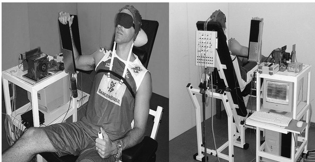
**Fig. 1.** The apparatus and participant position. The device was designed to passively move the arm in internal and external rotations about the shoulder joint.
